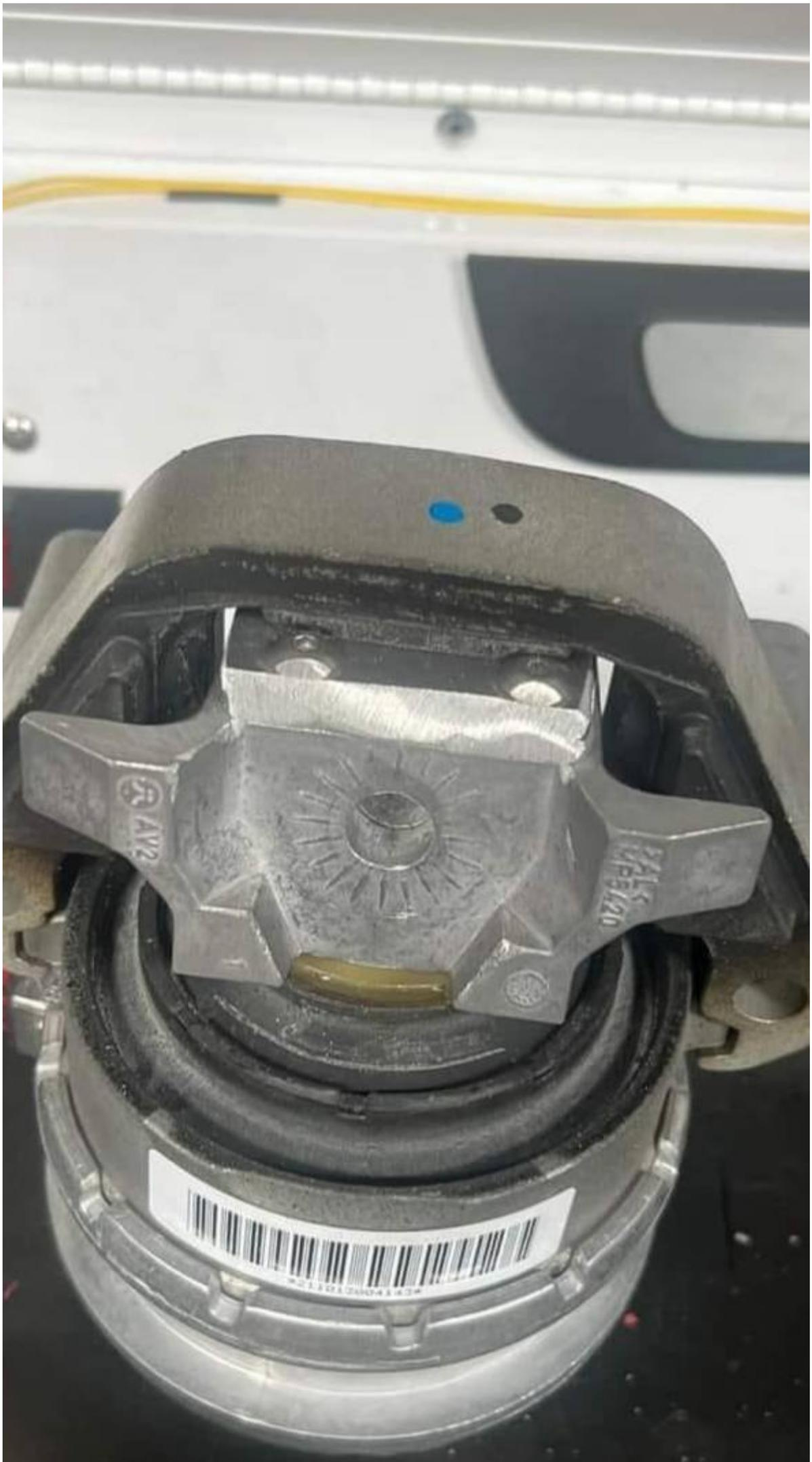
2. Use a syringe to inject [3M Window Weld](#)
